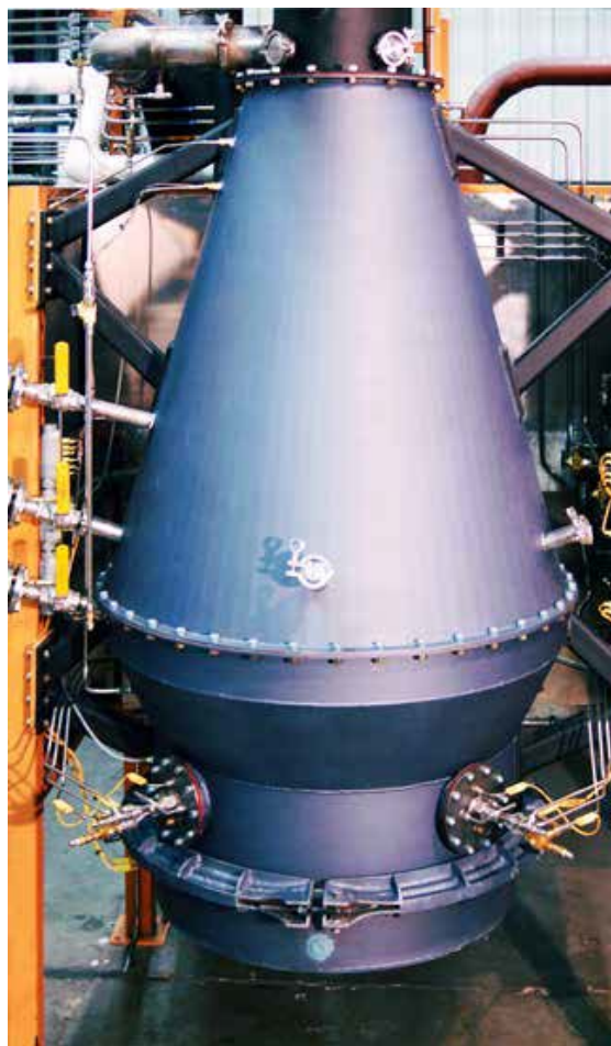
Figure 5-1 Sierra Energy FastOx™ Gasifier
